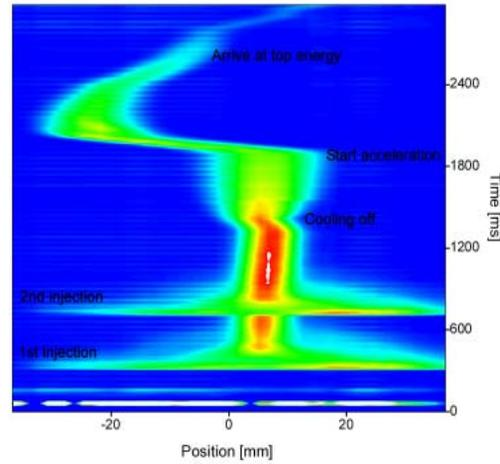
Figure 5: Horizontal cooling observed on the ionisation profile monitor.
