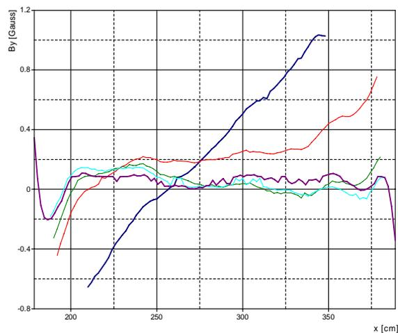
Figure 1: Adjustment of the cooler solenoid for the optimisation of the vertical field component. Five iterations (blue trace to magenta trace) were needed to reduce  $B_y/B$  to  $10^{-4}$  (for  $B = 1000$  G).
