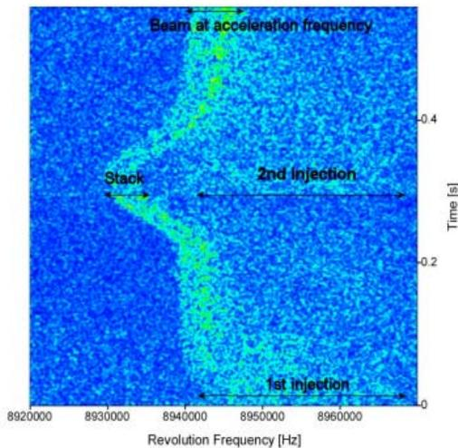
Figure 4: Longitudinal Schottky evolution showing the cooling and stacking of two injections of Pb ions.
