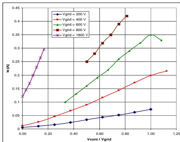
Figure 2: Electron beam current as a function of  $V_{\text{cont}}/V_{\text{grid}}$  for  $E_e = 2.5$  keV.
