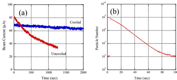
Figure 3: (a) Lifetime of the 7 MeV proton beam measured by DC-CT with and without the electron cooling when the average vacuum pressure is  $2 \times 10^{-8}$  Pa. (b) Lifetime of the 35 keV  $Mg^+$  beam measured by the electrostatic pickup when the average pressure is  $1 \times 10^{-8}$  Pa.
