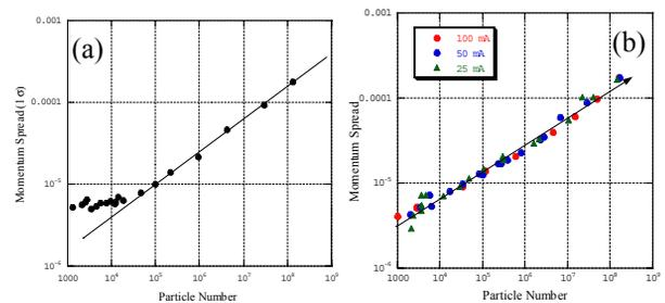
Figure 6: Measured momentum spread of the proton beam as a function of the particle number. The particle number was measured by the MCP residual gas monitor and the momentum spread was measured by the Schottky monitor. The voltage ripple of the cathode power supply is  $2 \times 10^{-4}$  (p-p) (a) and less than  $2 \times 10^{-5}$  (p-p) (b).
