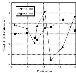
Figure 4: Closed orbit distortion of the cooled proton beam without corrections. The beam position is measured by the electrostatic pickup.
