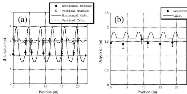
Figure 5: (a) Measured and calculated  $\beta$ -function in the ring. (b) Measured and calculated horizontal dispersion function in the ring.
