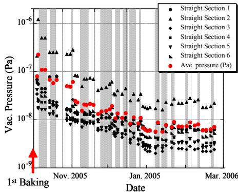
Figure 2: 5 months trend of the vacuum pressure after the first baking. There are 6 vacuum gauges in the 6 straight sections. The gray band shows the period of the operation.
