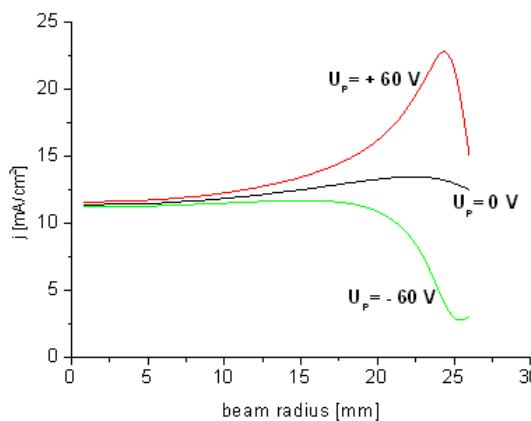
Figure 5: Various electron beam density profiles obtained by varying the Pierce electrode voltage.
