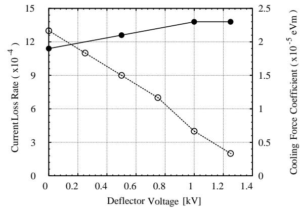
Figure 3: Reduction of the measured cathode loss current with applied electric field on the toroid electrostatic deflectors (white circles), while the longitudinal cooling force is almost unchanged (black circles).
