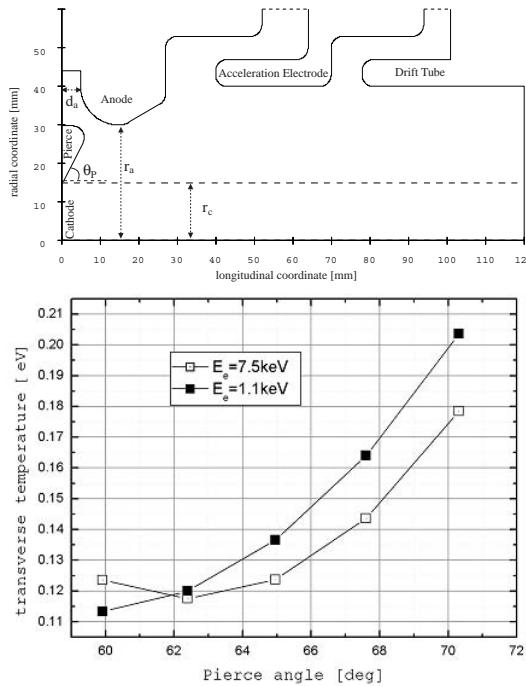
Figure 2: Up; schematic view of the electron gun, the cathode has a diameter of 30 mm and the Pierce electrode has an angle of  $\theta_P$ . Down; the transverse electron temperature is minimised for  $\theta_P = 62.9^\circ$ .
