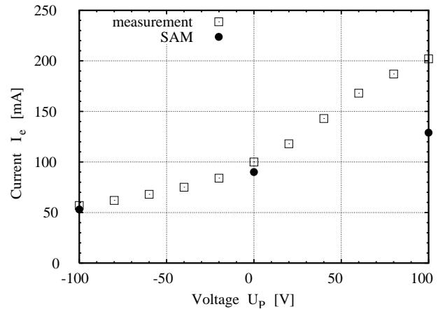
Figure 6: Dependence of the total electron beam current on the Pierce electrode voltage, and comparison with simulation with SAM code.
