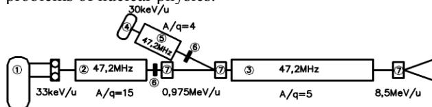
Figure 1: Scheme of the MILAC accelerator.
