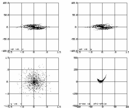
Figure 2: Radial phase portrait and output parameters of the beam at the accelerator output (LINACV2), number of macro particles is 10 000, input current is 40 mA, output current is 12 mA.
