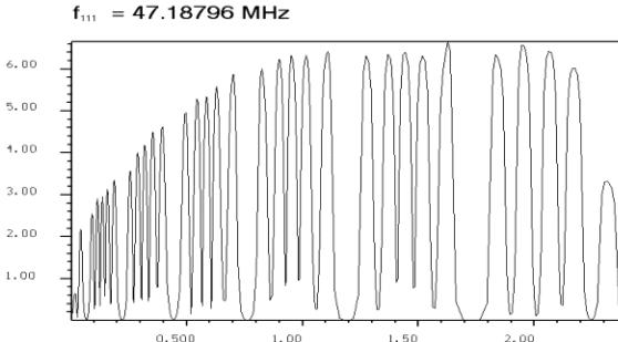
Figure 4: Distribution of the accelerating field along the gaps of the structure.
