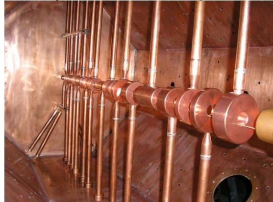
Figure 7: Photo of the internal view of the PSS-4 accelerating structure.
