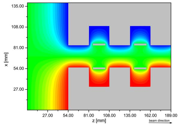
Figure 3: Potential distribution in the first cells of a 15 cell deflector.
