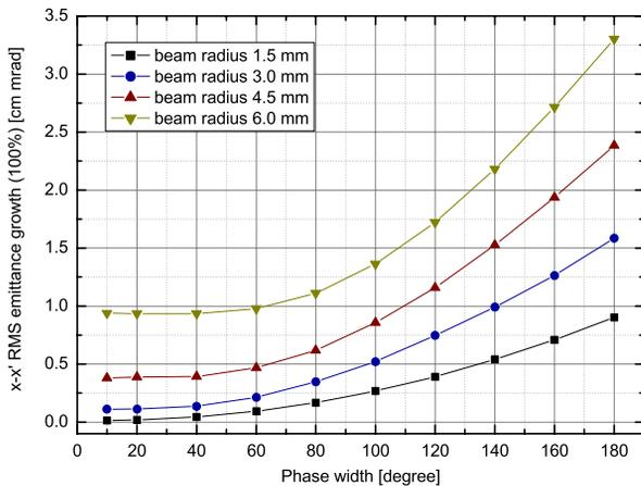
Figure 5: X-X' RMS emittance growth as a function of the phase width.
