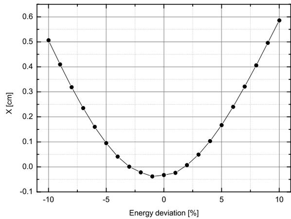
Figure 6: Divergence of the x coordinate of a stable particle as a function of the energy deviation.
