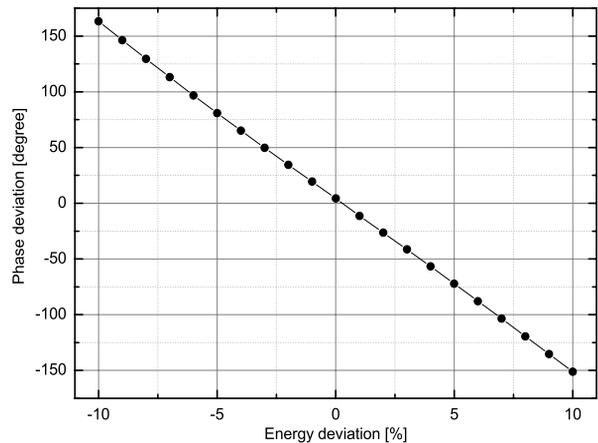
Figure 7: Phase divergence of a stable particle as a function of the energy deviation.
