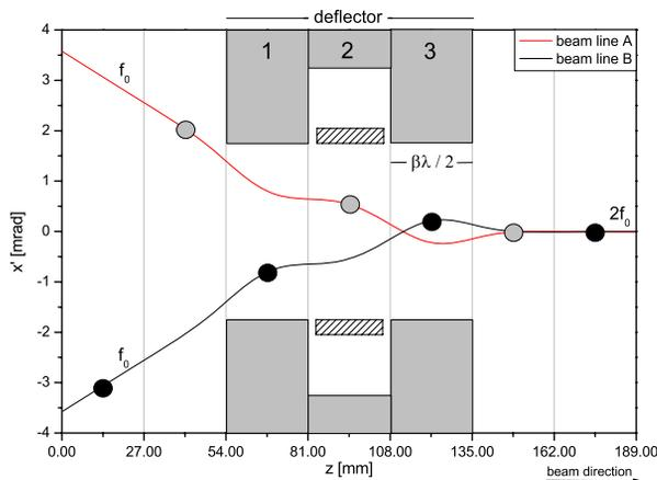
Figure 1: Schematic procedure of funneling.
