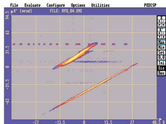
Figure 3: Emittance measurement with one beam line upgraded.
