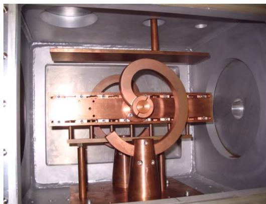
Figure 9: Structure in tank with tuning device.
