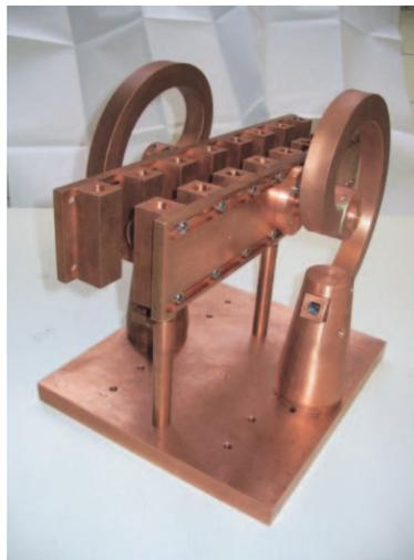
Figure 7: Photo of the new 15 cell funneling deflector.
