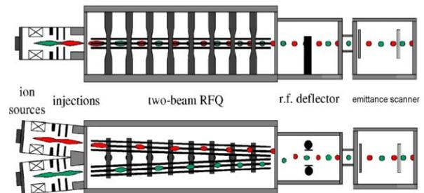
Figure 2: Scheme of the experimental setup.
