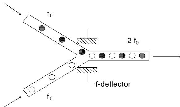
Figure 1: Principle of funneling.
