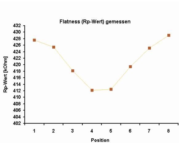
Figure 6: Flatness curve measurement.
