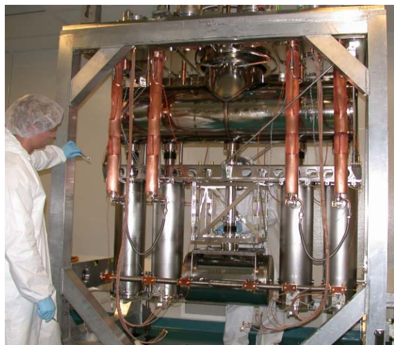
Figure 2: Cryomodule top assembly in the assembly frame prior to the cold test.
