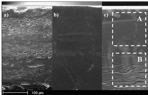
Figure 2 SEM images of sample cut by mechanical dicing saw: (a) as-diced; (b) after mechanical polishing; (c) after chemical etching.
