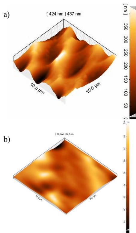
Figure 3: Atomic force microscopy images of silicon crystals after chemical etching under: a) the old methodology reported in Ref 7; b) the new methodology developed for the new experiment in the H8 CERN-SPS beam line.
