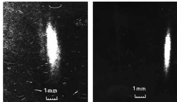
Figure 1: Image of the beam deflected through mechanically treated (left) and chemically polished crystals (right). The profile of the beam bent by a chemically polished crystal is more uniform and sharp (20  $\mu\text{rad}$  vs 100  $\mu\text{rad}$  at 70 GeV/c).
