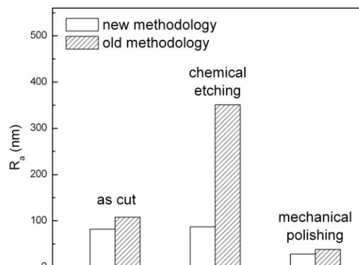
Figure 4: Quantitative analysis of AFM in terms of surface roughness of the crystal under different preparation methodologies; results from the old methodology (Ref. 7) are compared with results obtained with methodology applied for preparation of crystal for H8 beam line CERN-SPS experiment.
