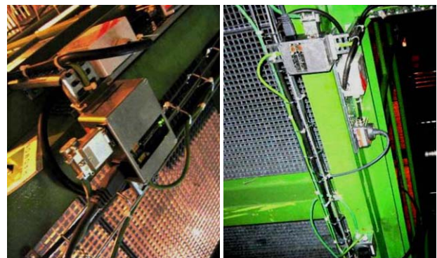
Figure 3: Radiation monitor installed in the UX85 area of the LHCb experiment.
