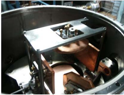
Figure 5. Pictured is one version of the quasi-optical pulse compressor which utilizes a four mirror configuration.
