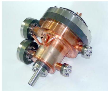
Figure 4. Pictured is the pulsed heating cavity which is awaiting installation onto one arm of the magnicon.
