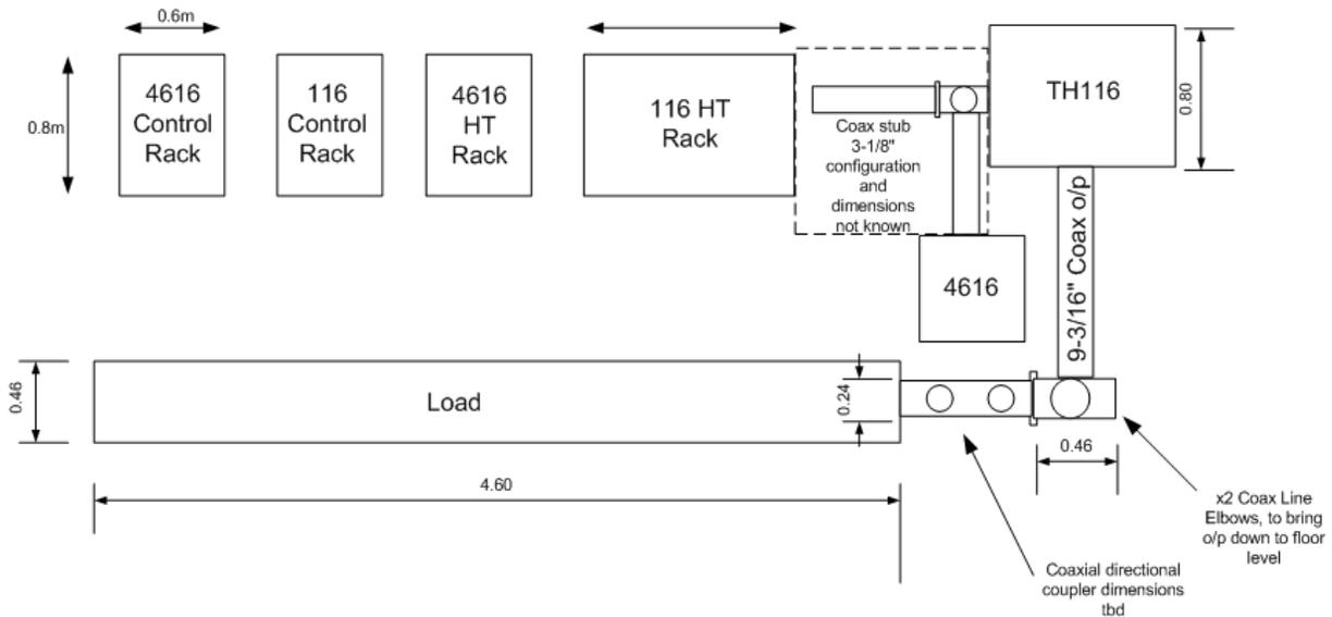
Figure 5: Proposed MICE RF test stand layout
