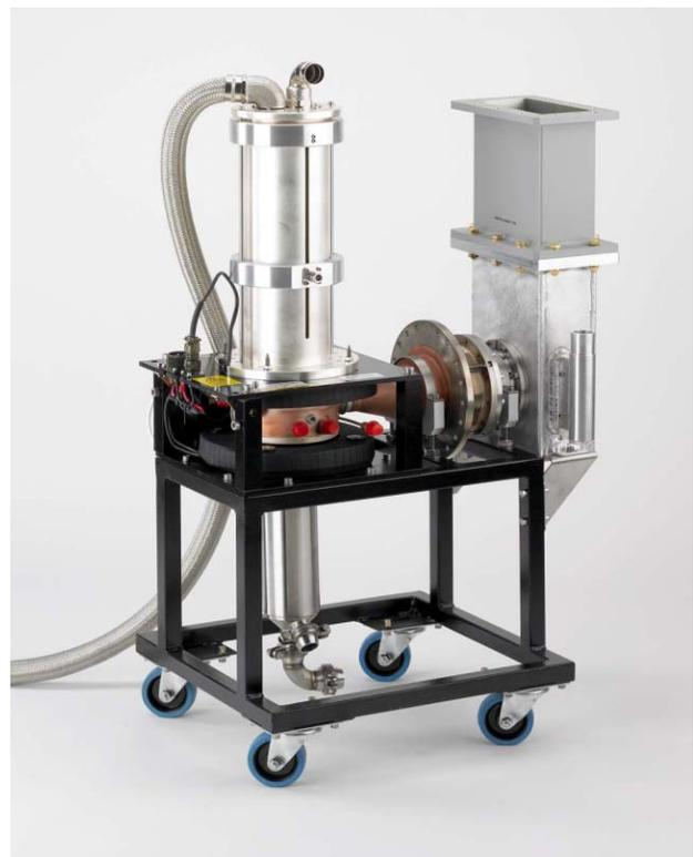
Figure 1: 1.3GHz IOT in its circuit
