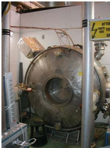
Figure 4: The 88 MHz test cavity.
