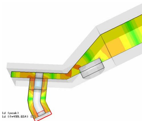
Figure 5: CST MICROWAVE STUDIO® simulation of WATRAX.
