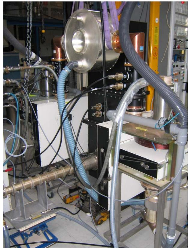
Figure 3: CaCo under high power test at TED.
