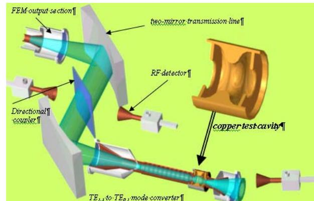
Figure 1: Scheme of 30 GHz experimental set-up.
