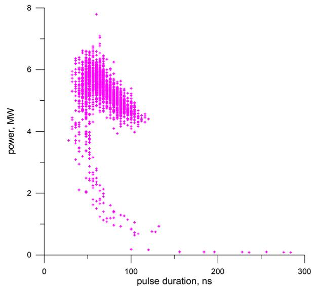
Figure 5: Statistical distribution of the transmitted RF pulses.
