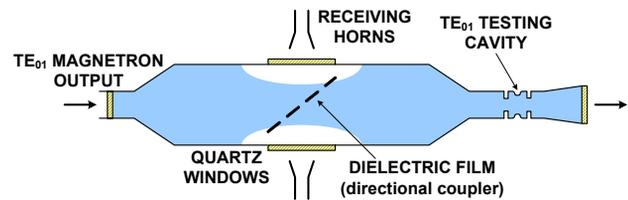
Figure 8: Scheme of 36 GHz experimental set-up.
