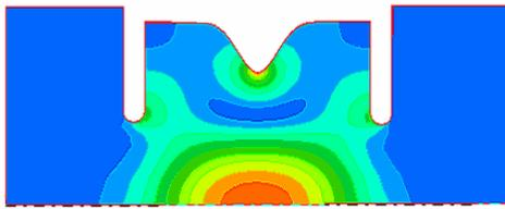
Figure 7: Magnetic field distribution at new TE<sub>011</sub> test cavity.
