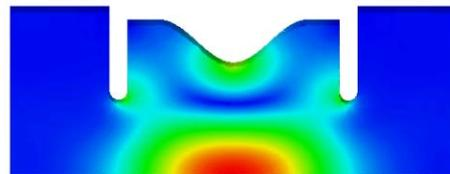
Figure 2: Magnetic field distribution at the used  $TE_{011}$  test cavity.
