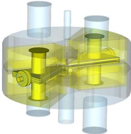
Figure 1: Basic model of KIRAMS-30 RF system.
