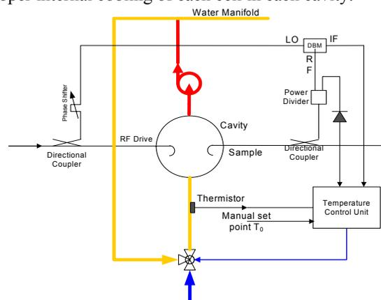
Figure 3: Small deviations of RF drive with respect to sampling signals result, through a temperature control unit, to an error signal activating an automated mixing valve to optimized temperature of each cavity independently.
