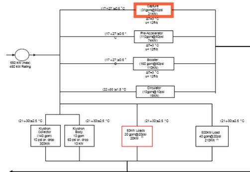
Figure 1: Main cooling system schematic.
