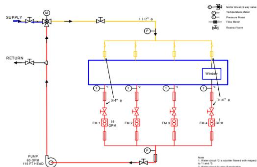
Figure 2: The mixing of cold and heated water for one of the structures and associate monitoring devices.
