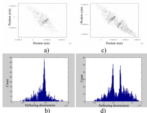
Figure 7: Image of single femto second electron bunch (a) and its histogram (b) Image of two femto second bunch separated (c) 5ps and its histogram (d).
