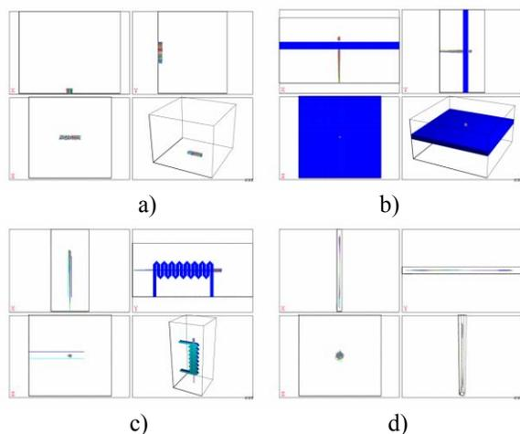
Figure 6: Electron trajectory from simulation a) electron ejection from cathode b) electron accelerated by static field c) electron deflected by the meander line field d) electron focused by solenoid field.
