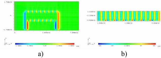
Figure 4: a) longitudinal field(V/m) of meander line (vertical offset 0.2mm). b) center part of a).
