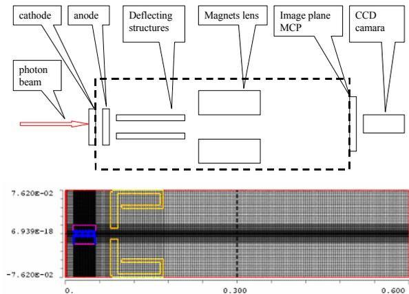
Figure 1: schematic of streak camera and Top view of the MAFIA model.
