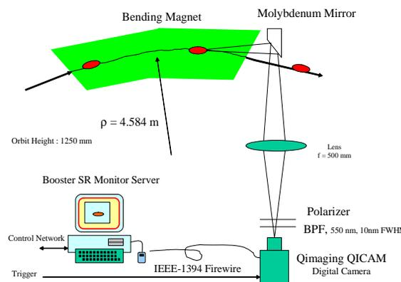
Figure 1. System block diagram of the booster synchrotron radiation monitor.
