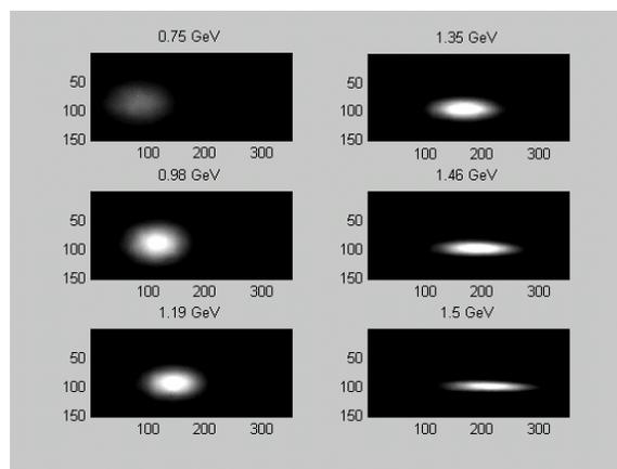
Figure 2. Example of observed beam profiles during ramping with various energies. With 2x2 binning, the pixel size is 9.4  $\mu\text{m}$  x 9.4  $\mu\text{m}$ . Exposure time is 0.5 ms.
