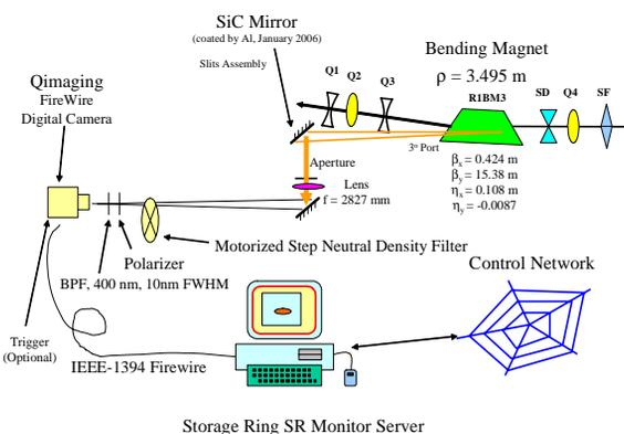
Figure 4. Optics of the synchrotron radiation monitor in the storage ring.
