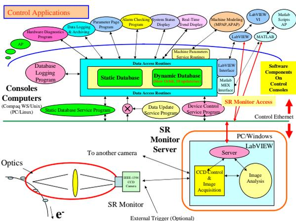
Figure 3. Synchrotron radiation monitor software system.
