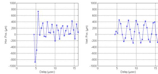
Figure 7. Variation of beam profile centroid just after injection kicker fired. Stored beam performed betatron oscillation in horizontal (left side) and vertical plan (right side).
