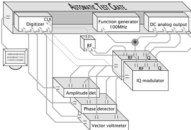
Figure 2: Automatic test set-up.
