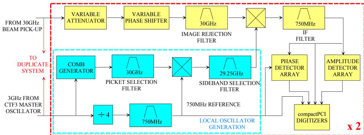
Figure 5: System for tests with beam in CTF3.
