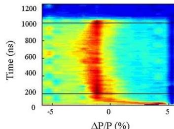
Figure 7: Energy spectrum for a 1μs long pulse. Beam energy is 73 MeV and FWHM energy spread is 1.8%
