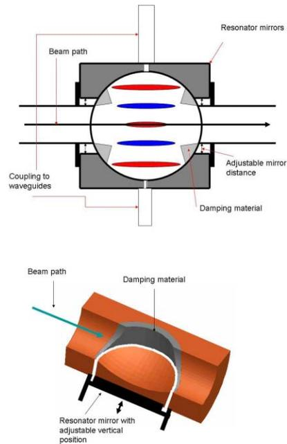
Figure 7: Artistic views of the nearly-confocal resonator pick-up to be installed in CTF3.
