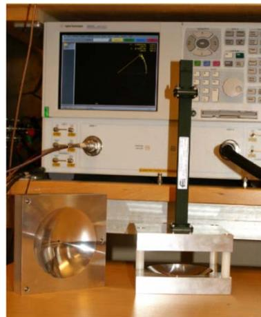
Figure 4: Open nearly-confocal resonator prototype with its extraction waveguide. One Aluminium plate with its mirror cavity is also shown.
