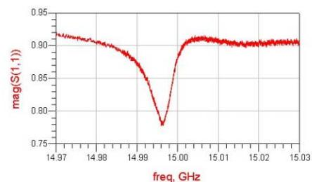
Figure 2:  $S_{11}$  versus frequency for the confocal resonator under-critically coupled to a waveguide. The input port is the coaxial transition to the waveguide.
