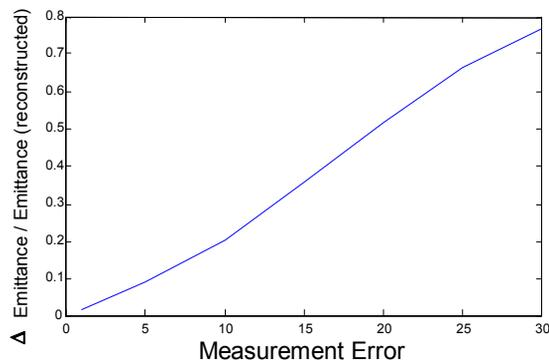
Figure 4: Measurement error vs. projected emittance
