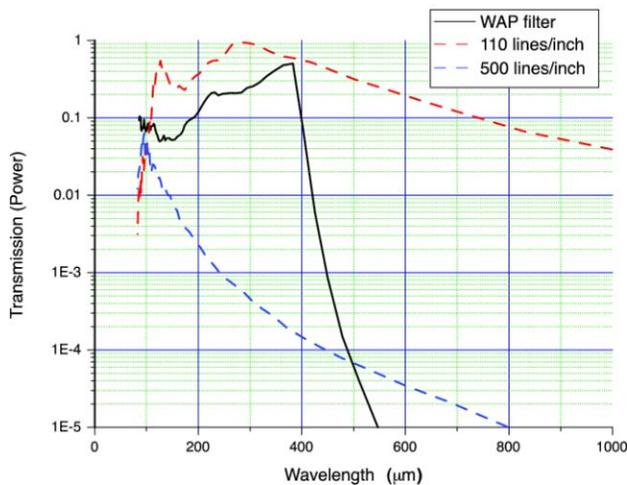
Figure 5: A comparison of power transmission characteristics of a WAP filter (solid line) and two wire mesh filters (dashed lines). Note the steep cut-off of wavelengths by the WAP filter after its designed wavelength, compared to the gentle slopes of the wire mesh filters.
