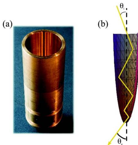
Figure 4: (a) A brass non-imaging light concentrator as used in this experiment, (b) light reflecting through the concentrator.
