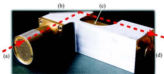
Figure 3: The assembled optical system, and the path of radiation passing through it. Shown are (a) the WAP filter and its holder, (b) a  $45^\circ$  plane mirror, (c) a non-imaging light concentrator, and (d) the position of the detector, when attached to the optical system.
