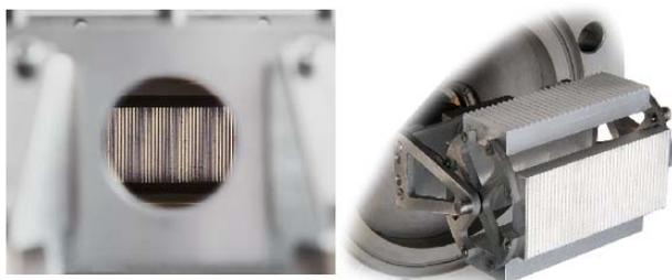
Figure 2: The ‘carousel’ containing 3 aluminium gratings with different periodicity, and one blank piece with the same dimensions. The carousel can be rotated by  $90^\circ$  during the experiment, and enables a quick turn-around of results.
