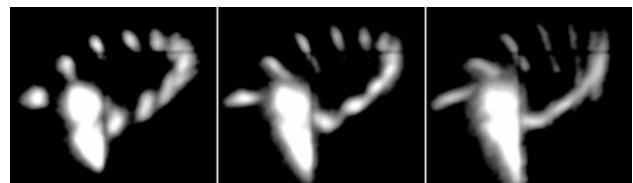
Figure 5: Matching with synchrotron radiation of RTM2: The main area contains the first 40 turns, turn 41 is deflected to separate the following turns using the betatron motion. Matching gets worse from left to right to demonstrate the usage ( i < 10 nA).
