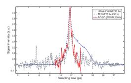
Figure 3: Square of beam profiles measured by spectral decoding (EO-SD) with a not optimized setup, and spatial decoding (TEO). Both use a  $180 \,\mu m$  GaP-crystal. Blue: LOLA with lowest streak (29.6 fs/px).
