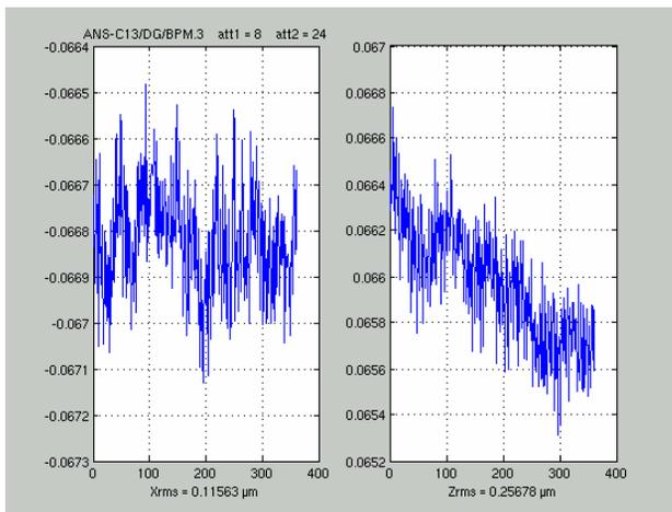
Figure 4: Libera noise in Slow Acquisition mode:  $X_{rms} = 0.11\mu\text{m}$ ,  $Z_{rms} = 0.25\mu\text{m}$  (360 acquisitions in 180 s).
