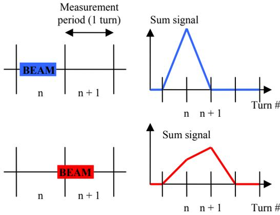
Figure 1: One-turn Sum signals on two BPMs with different phases of the beam with respect to the Machine Clock (MC).
