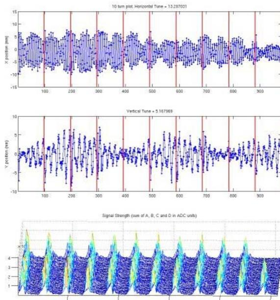
Figure 2: Multiple turns (>20) with injection kickers. The vertical lines in the plots above indicate a revolution. Top: Horizontal position ( $v_x = 13.21$ ). Middle: Vertical position ( $v_y = 5.17$ ). Bottom: sum signal where each line represents a turn.
