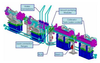
Figure 5: Integration study for ring collimators with all required infrastructure in the LHC tunnel.
