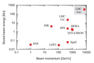
Figure 1: Stored beam energy versus beam momentum for various past, present and future high power accelerators.
