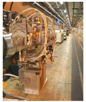
Figure 6: Photograph of an installed ring collimator on its quick plug-in support in IR8 of the LHC.
