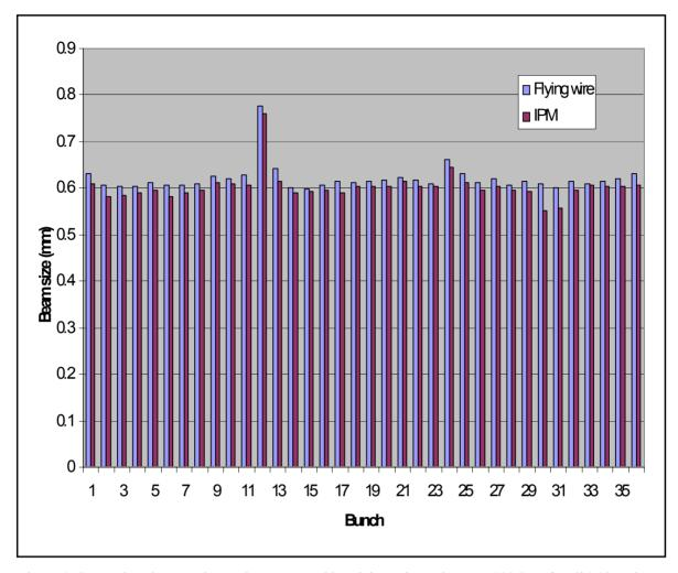
Figure 6: Comparison between beam sizes measured by Flying Wire and IPM at 980GeV, for all 36 bunches. The difference in ratio for bunches 30 and 31 is a known problem with the IPM electronics, causing the revolution marker to couple into the input signal.
