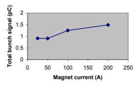
Figure 4: Measured beam size (top) and total signal (bottom) as a function of magnet current. 200A correspond to the nominal field of 0.2T.
