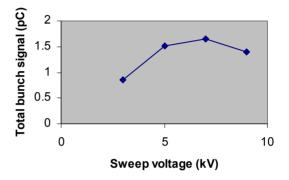
Figure 5: Measured beam size (top) and total signal (cyan) as a function of sweep voltage. 7kV correspond to a electron kinetic energy of about 3keV.
