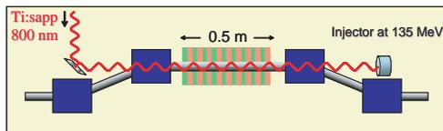
Figure 4: Scheme of laser heater (LCLS)[16]
