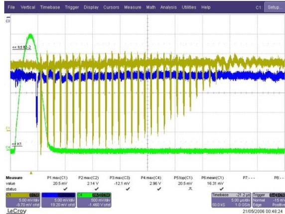
Fig. 3: successive turns detected by the FCT without RF and with sextupoles OFF.
