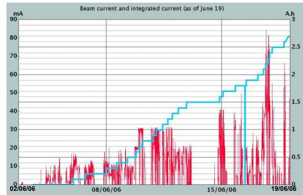
Fig.4: Beam current (red) and evolution of the integrated current (blue) during the 3 week run.
