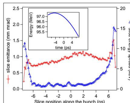
Figure 5: Slice emittance (red line) and slice energy spread (blue line) along the ramp medium bunch calculated at the exit of the photoinjector. Inside plot: Longitudinal phase space including longitudinal wakes. Head is on the left.
