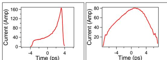
Figure 4: Ramping current distribution at the cathode (left) and at the injector exit (right), for a 800pC bunch.
