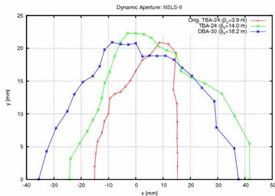
Figure 3: Dynamic Aperture (normalized with  $\sqrt{\beta_x \beta_y}$ ) for the Original TBA-24, TBA-24, and DBA-30 Options.
