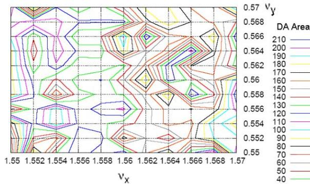
Figure 1: Tune Scan of Normalized Dynamic Aperture for the Original TBA-24 Cell.
