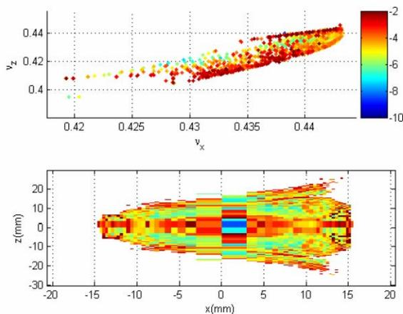
Figure 2: Frequency Map<sup>5</sup> for the Original TBA-24 Cell ( $\beta_x = 3.0 \text{ m}, \beta_y = 5.5 \text{ m}$ ).
