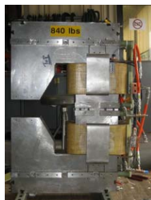
Figure 6: Prototype chicane dipole magnet .
