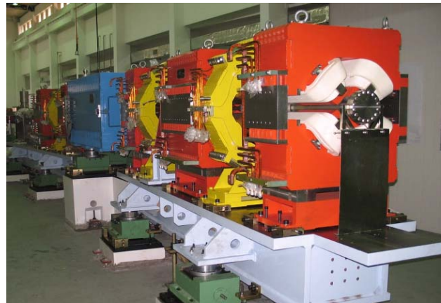
Figure 2: A mechanical sector of the SSRF storage ring
