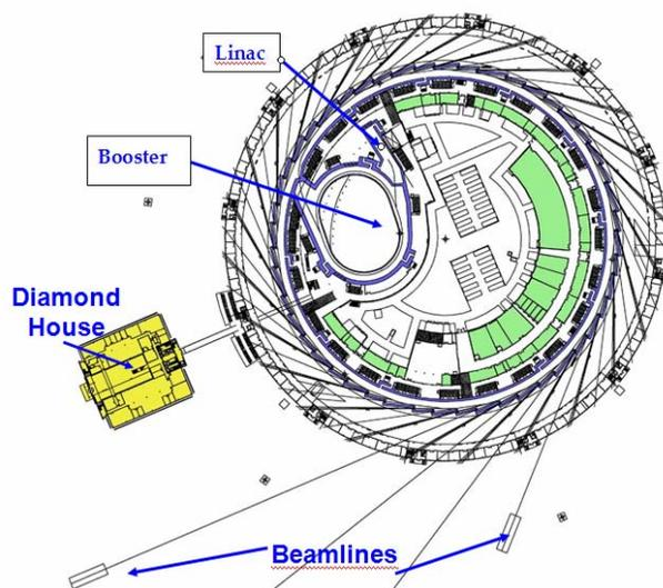
Figure 1: Layout of Diamond Light Source
