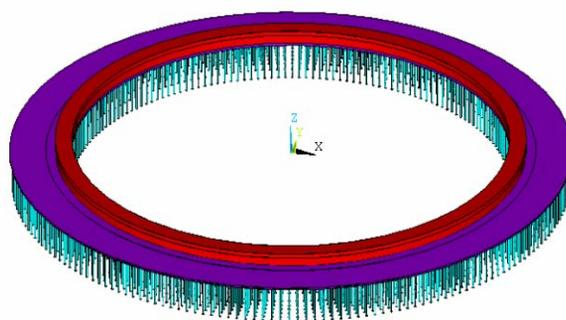
Figure 3: FE model of slab with piles
