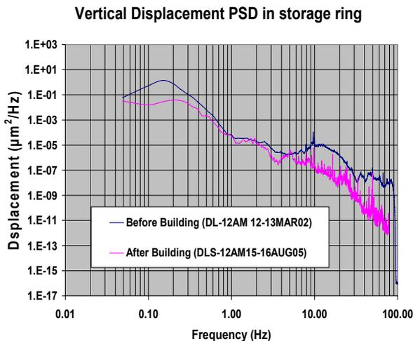
Figure 2: Ground PSD before and after DLS construction
