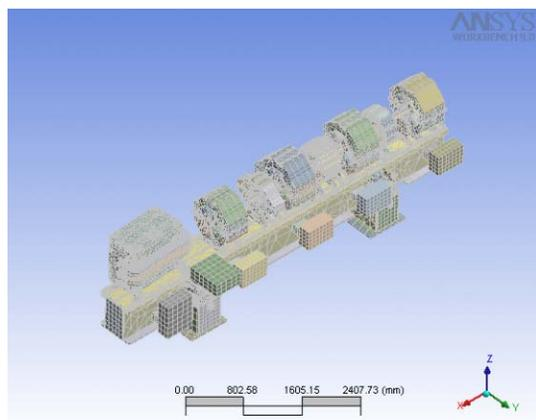
Figure 5: FE mesh for Girder 2
