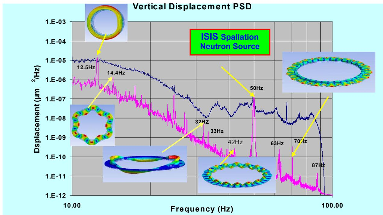
Figure 4: Natural frequencies and modal shapes of foundation slab in Diamond Light Source.
