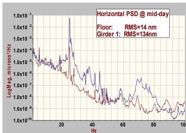
Figure 6: Horizontal PSD of Girder 1 (upper) and floor
