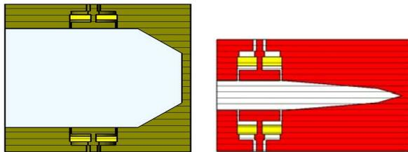
(a) Cross section of the arc beam pipe as modeled (half) with the upper and lower BPMs. (b) Cross section of the narrow beam pipe as modeled (half) with the upper and lower BPMs.
