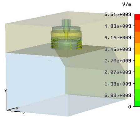
Figure 3: Electric field distribution of the mode at 9.035 GHz.
