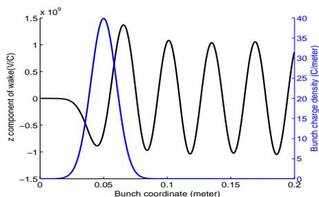
Figure 6: Longitudinal (z) component of the wake potential along the bunch coordinate (s) for BPMs in the narrow beam pipe.
