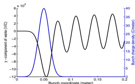
Figure 7: Transverse (y) component of the wake potential along the bunch coordinate (s) for BPMs in the narrow beam pipe (transverse beam offset 2.0 mm).
