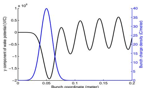
Figure 5: Transverse (y) component of the wake potential along the bunch coordinate (s) for BPMs in the arc beam pipe (transverse beam offset 5.0 mm).
