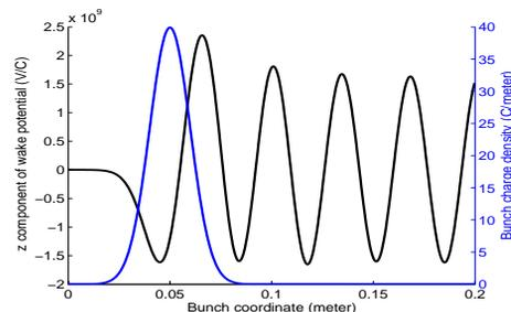
Figure 4: Longitudinal (z) component of the wake potential along the bunch coordinate (s) for BPMs in the arc beam pipe.
