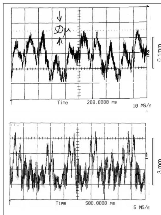
Figure 2: Oscilloscope traces showing 0.1 mm changes at 20Hz measured at a certain BPM at  $f_s=1.3$  kHz (upper screen) and 3mm jumps at 44Hz modulation at  $f_s=0.3$  kHz (lower screen)
