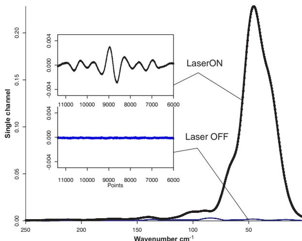
Figure 3: Typical raw interferograms and rapid-scan FTIR spectra measured at 4 mA bunch current during a regular femtoslicing shift. The acquisition time is 3 s at 10  $\text{cm}^{-1}$  spectral resolution.
