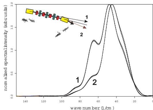
Figure 5: Comparison of normalized THz spectra from upstream and downstream dipole after the slicing section. The inset indicates that a shorter longitudinal density modulation is expected at the upstream dipole which is  $5.2 \text{ m}$  closer to the modulator.
