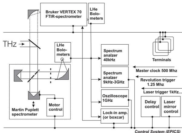
Figure 2: Instrumentation, detection- and trigger schemes for time-resolved spectral characterization of laser-induced coherent THz pulses at BESSY.
