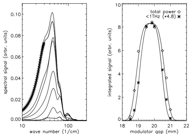
Figure 4: Evolution of rapid-scan THz spectra (left) while detuning the resonance in the modulator. Two resonance curves from different integrated parts of the spectra are also shown (right).
