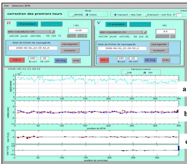
Figure 2: Result of the first turn trajectory correction. a: intensity seen by each of the 120 BPMs. b: beam positions after the first turn correction c: correctors values (H in red and V in blue).
