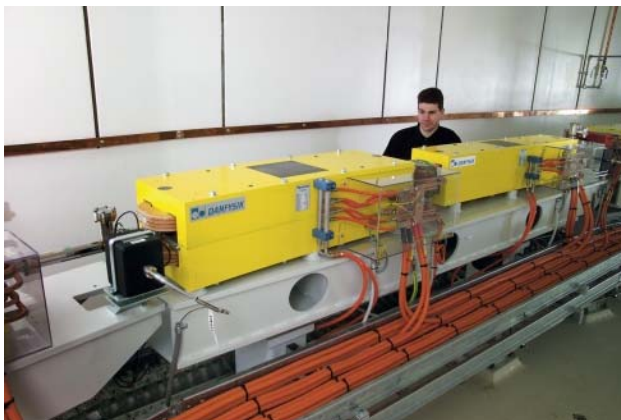
Figure 3: BD and BF magnets placed on a common girder
