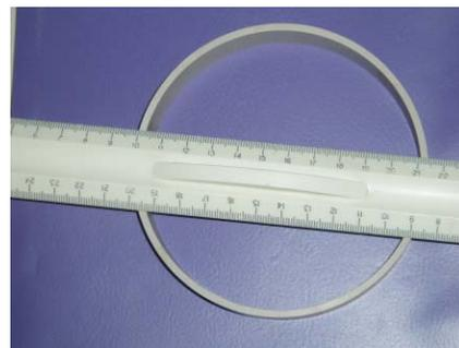
Figure 1: Large-diameter ceramic ring sample made of BST-MgO (BSM) ferroelectric. The ring diameter is of 110 mm and the ring thickness is of 2.8 mm.
