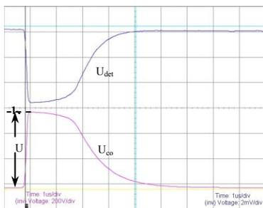
Figure 2: Typical time profiles of the control (biasing) pulse voltage and the BSM ferroelectric response after detection.
