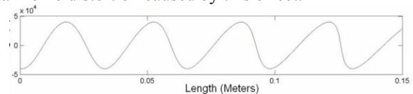
Figure 7: FDTD simulation of the nonlinear line.
