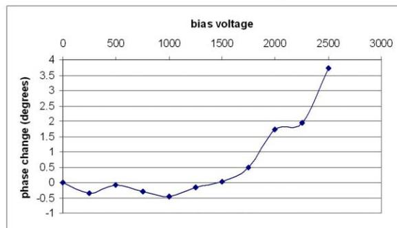
Figure 6: Observed phase change at 468 MHz.
