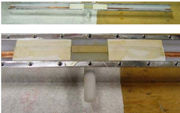
Figure 5: Prototype phase shifter showing BST bar (center) surrounded by two alumina matching sections with hole in center for DC feed.
