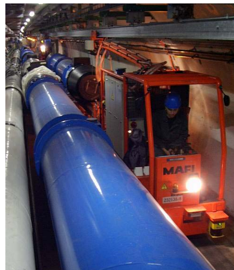
Figure 1: Limited space for the magnet transport in the LHC tunnel
