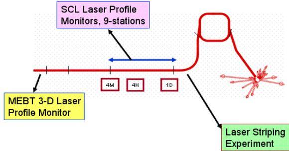
Figure 1. Longitudinal profile monitor located at 2.5 MeV MEBT uses a Ti-Sapphire laser phased locked at 1/5 RF bunching frequency [402.5 MHz]. Nine SCL profile monitors and the laser stripping stations use one Nd:YAG laser.
