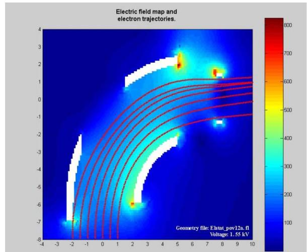
Figure 4. Trajectory of the liberated electrons into MCP is modeled by Victor Alexandrov from BNIP.
