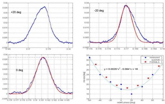
Figure 5. Longitudinal bunch profile measured with mode-locked laser in the MEBT (blue dots) and Gaussian fit (red line). RMS bunch-length vs. the rebuncher phase (measurements – squares, simulation – stars, solid line quadratic fit) are shown on bottom right figure.
