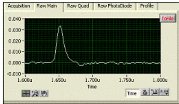
Figure 7. Liberated electrons are collected by the Faraday cup shows the direct measurement of signal at each step of generation the transverse profiles.
