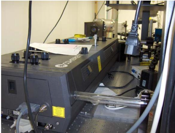
Figure 2. Ti-Sapphire mode-lock Laser with 2 Pico-second pulse length is used to measure the longitudinal bunch length at 2.5 MeV.
