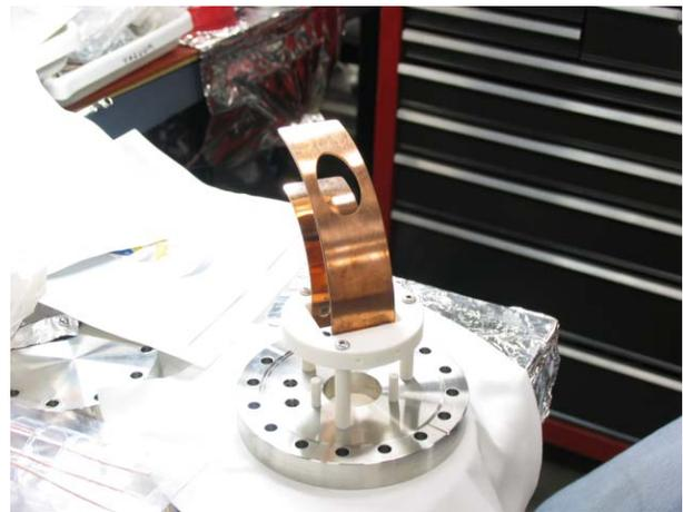
Figure 3. Copper electrostatic deflectors mounted on Al<sub>2</sub>O<sub>3</sub> insulators are biased to ~+/-800 Volts on two plates. MCP is not shown in this picture.
