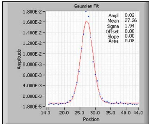
Figure 8. The blue dots are baseline subtracted integral of the figure (7) above. The Gaussian fit is shown in Red.
