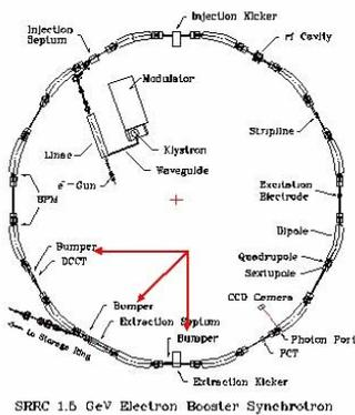
Figure 5: Layout of TLS injector. The bumpers are located at sections 8, 9, 10.
