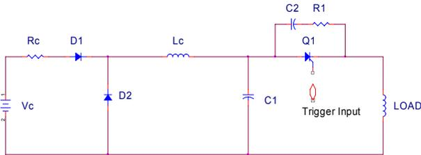
Figure 2: The charging voltage at  $C_1$  is determined by  $V_c$  of the command charging PS. Resistor  $R_c$  and a small inductor  $L_c$  are added for practical reasons.
