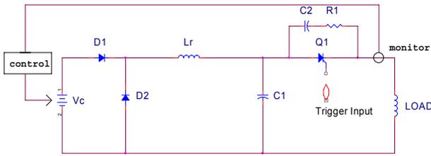
Figure 1: The large inductor  $L_r$  acts for resonant charging to multiple the voltages at capacitor  $C_1$ . The load monitor provides feedback information for precision control of the magnet current.
