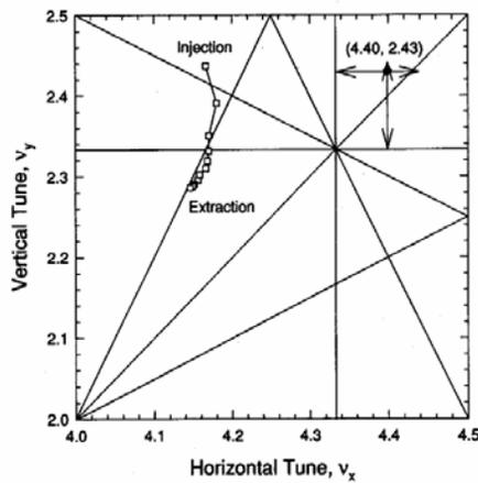
Figure 4: Tune diagram of the booster. The design tunes ( $v_x = 4.40, v_y = 2.43$ ) and corresponding tuning ranges for 50 MeV, DC mode operation are shown in the upper-right corner. Tune drift in ramping operation is also indicated.
