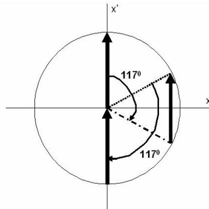
Figure 6: Phase space evolution of the electron beam at extraction moment in TLS booster ring.
