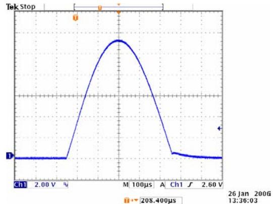
Figure 3: Example of the pulsed current signal of extraction septum. ( pulse width : 500  $\mu$ s; pulse height : 1000 A / 2 V )
