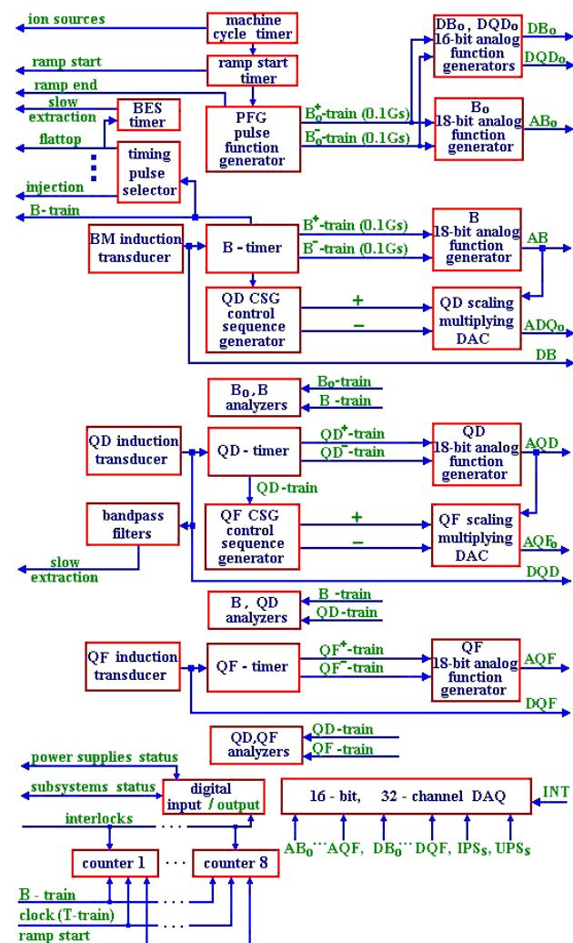
Figure 1: Schematic diagram of the MPSC.
