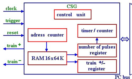
Figure 3: Block diagram of the CSG.
