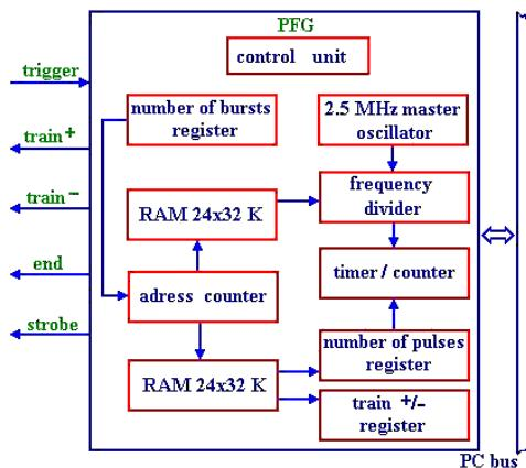
Figure 2: Block diagram of the PFG.
