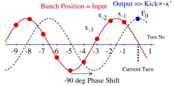
Figure 2: The required response of the FIR filter. The one-dimensional case is shown. The phase shift between the input and the output should be -90 degree.
