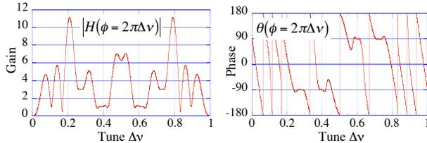
Figure 3: Frequency response of the 20-tap FIR filter for single-loop two-dimensional feedback for the PF ring. Horizontal tune  $\Delta v_x = 0.6$  and vertical tune  $\Delta v_y = 0.28$ .
