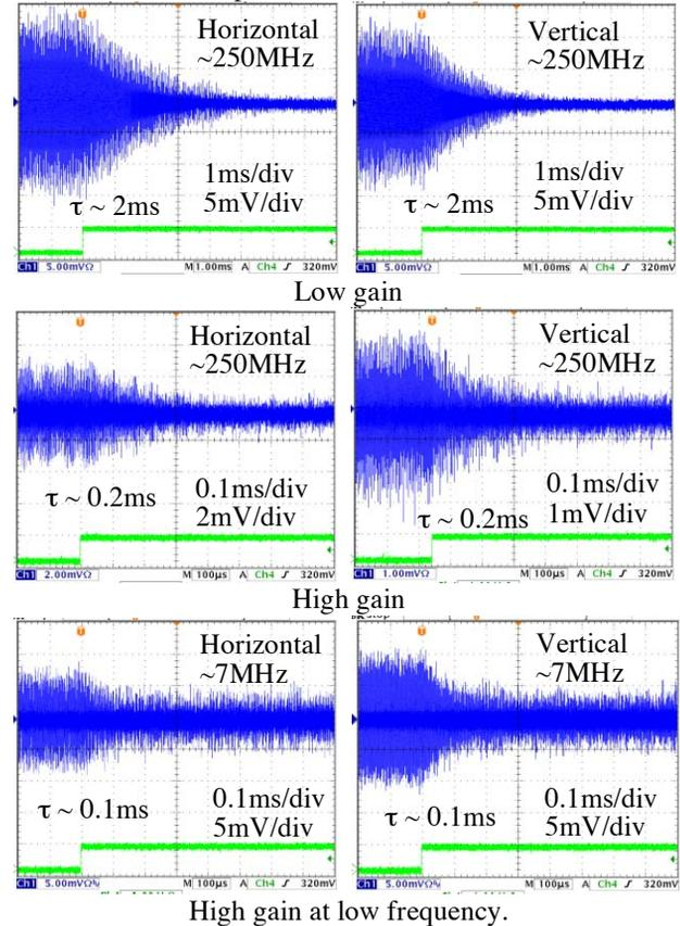
Figure 4: The damping of oscillation excited by external forces under the feedback ON with lower gain and higher gain. The forces are turned off when gate signals in the lower traces shift high. The directions and frequencies of the forces and damping time  $\tau$  are shown in the figures.
