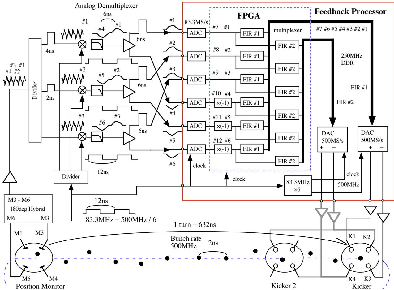
Figure 1. Block diagram of the single-loop two-dimensional feedback system for the Photon Factory ring. Currently two kicker electrodes connected FIR #1, K1 and K3, are used for feedback. Lines for the electrode K2 and K4, and lines for Kicker 2 show optional schemes that are enabled by using another stream of FIR filter (FIR #2).
