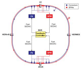
Figure 3: Layout of the local IP orbit feedback of HERA.
